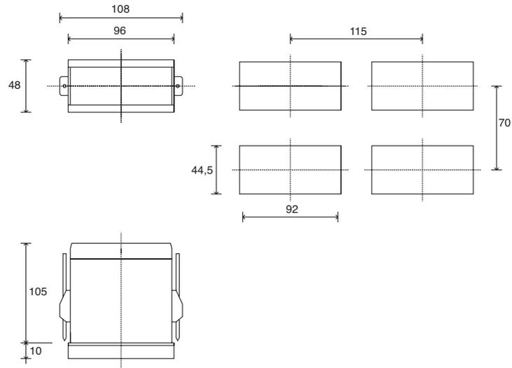
Dimensions: 96x48mm (1/8DIN), depth 105mm
