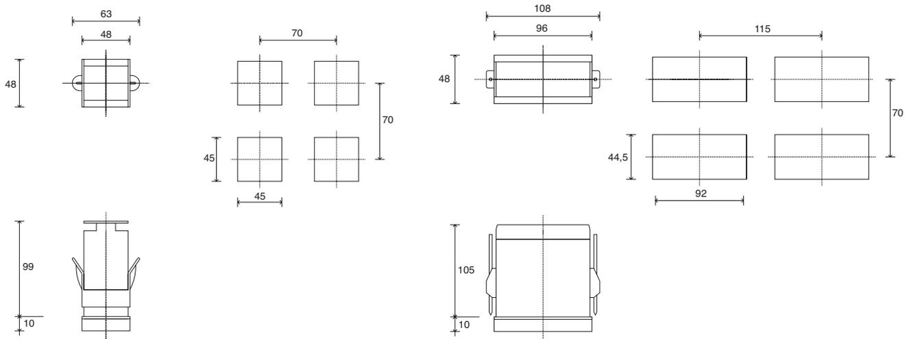
Dimensions: 48x48mm - 96x48mm (1/16DIN - 1/8DIN), depth 99mm - 105mm
