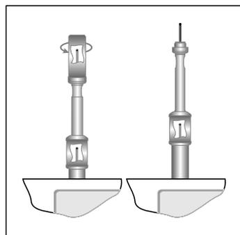
Fig.2 Hot-wire probe mod. HD2001.2.
