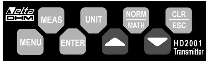
**MEAS** By repeatedly pressing this button the main variable displayed in the first line of the display can be selected. This function is cyclic: %RH >> Barometric Pressure >> Wind speed (for the HD2001.2 model) >> %RH...
