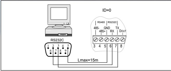
Fig.5 Connection to PC/ device with RS232C protocol.
