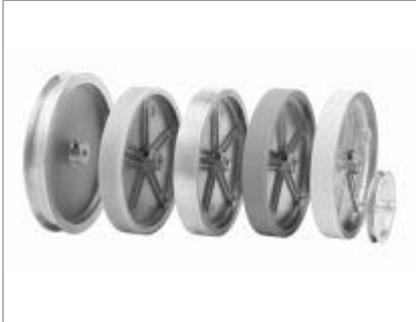
In order to prevent the result being distorted when the shaft encoder is driven by a measuring wheel make sure that the slip is as small as possible. When selecting the tread (surface), take into account the structure, stretchability, thickness, and resistance to being carried along of the material being measured.
