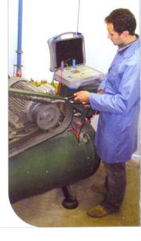
TeraOhm 10 kV is a professional diagnostic insulation tester, which allows measurements on high voltage rated equipment. It is specially well suited for:
